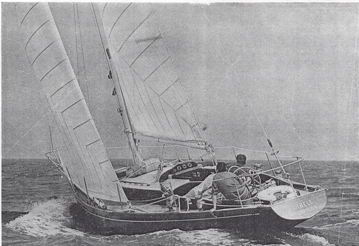
Swan's sistership Cybele shows to advantage in this quarter shot. Swan 36 will have tiller steering, wooden spars and is built in fibreglass.
