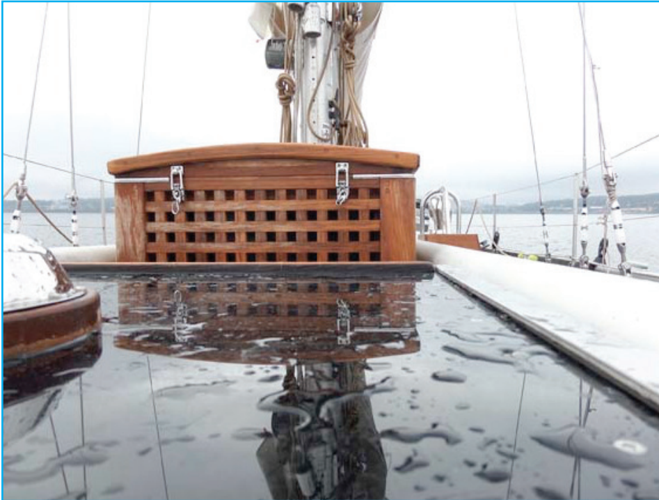
Hill's solution to tender storage, constructed by himself. It can be removed easily when in racing mode.
