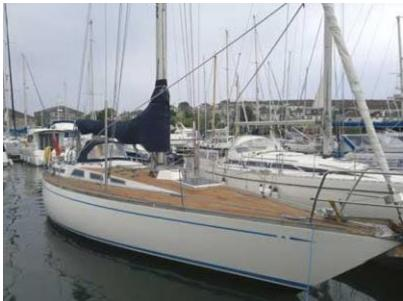
No doubt experts will correct me if I'm wrong, but I believe the 38 was the first of the Swans to sport the signature, low, slope-sided, coachroof wedge which seems to grow out of the deck and merge into the cockpit coaming, and which, for a time, became a characteristic feature of the marque, until it was copied by many other designers. This feature makes the decks appear wider and allows excellent forward visibility from the cockpit.
