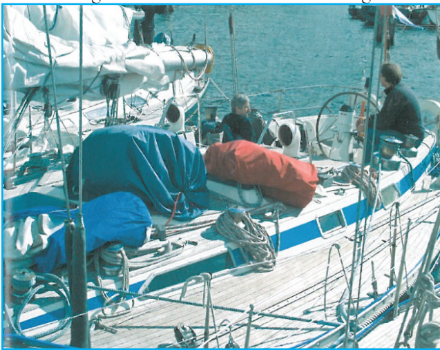
The deck has an overlay of teak battens and is dominated by a large number of winches
