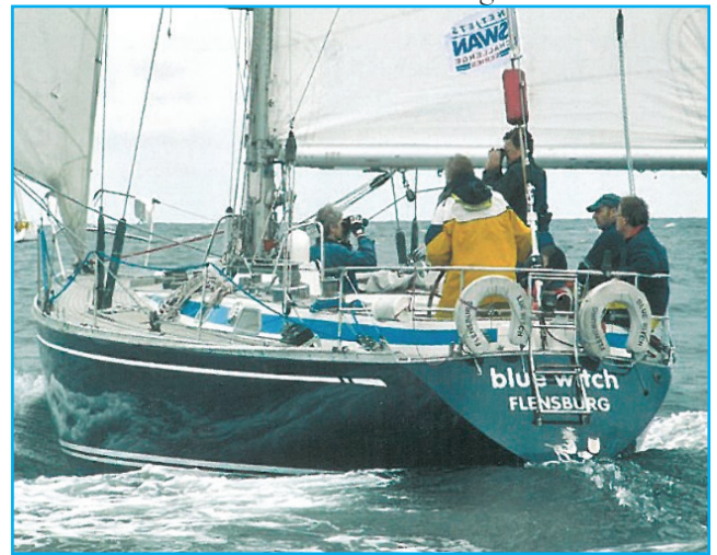
Because of mid-boom sheeting the operation of main sheet and traveller is tiring
