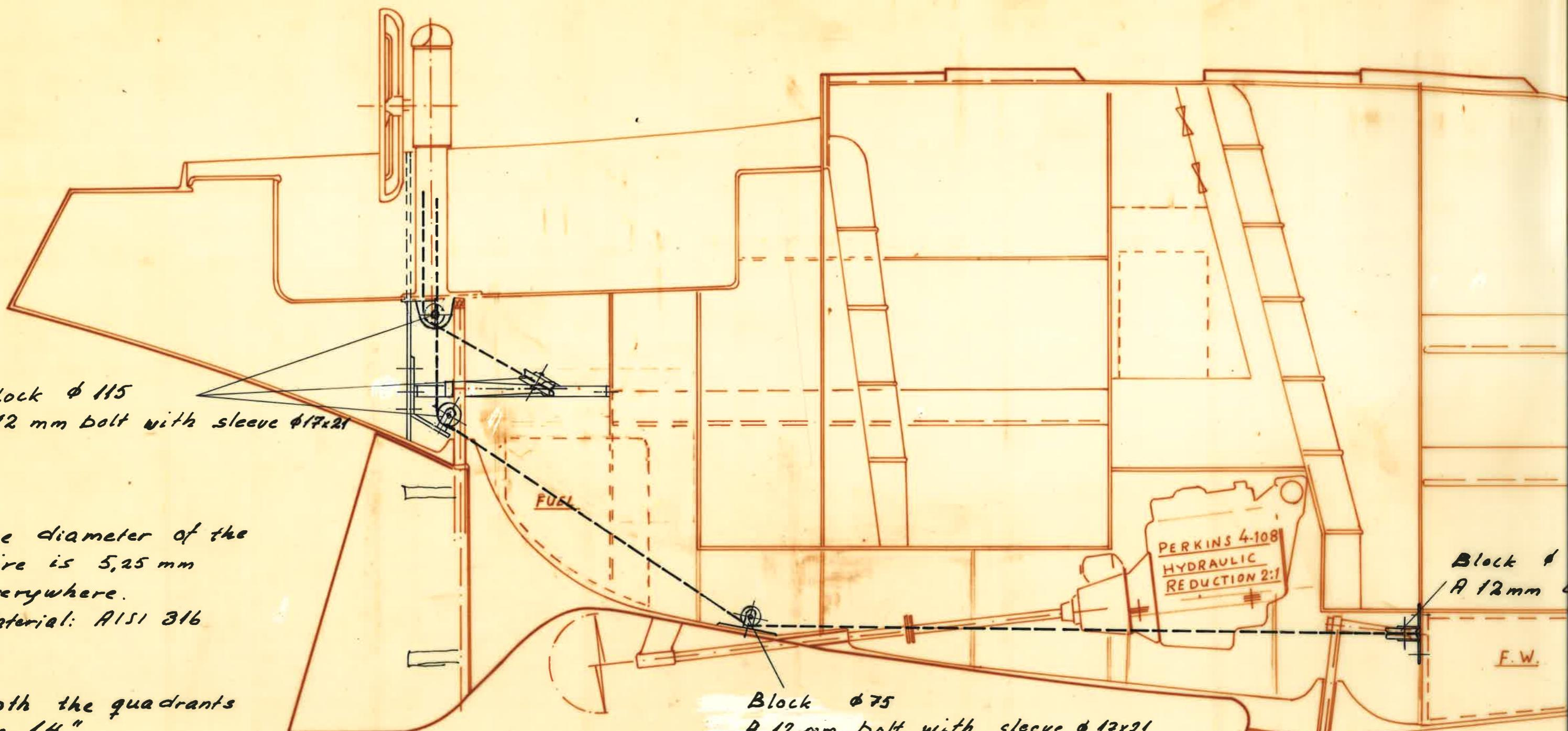
The main rudder turns  $35^\circ + 35^\circ$
