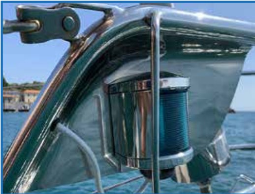
39 - Nav lights are Hella Marine, and on most S&S Swans are very well protected by a stainless steel shell
