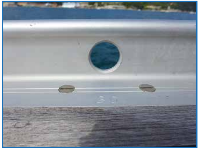
36 - Nautor built toerail, anodized aluminum, with numbered drilled holes and fairleads, and all perfectly aligned screws. Sometimes toerail could appear a bit worn, pay attention because it may just be an insignificant cosmetic problem. They are built to last forever
