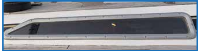
33 - Original window frames on S&S Swans are GRP, and painted to seem aluminum
