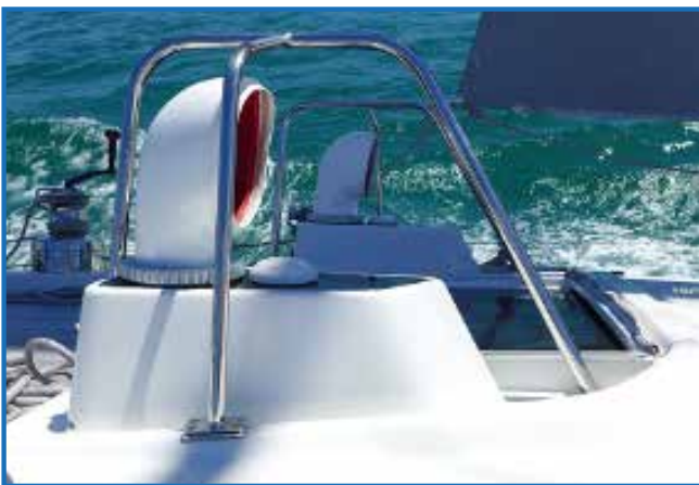
29 - Dorade Box, originally designed by Olin J. Stephens (Type plan D10)
