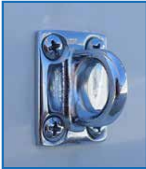
52 - Chromed bronze Nautor built padeye, on deck to fix sprayhoods laces, and down below to fix kitchen belts, chart table belts, etc.
