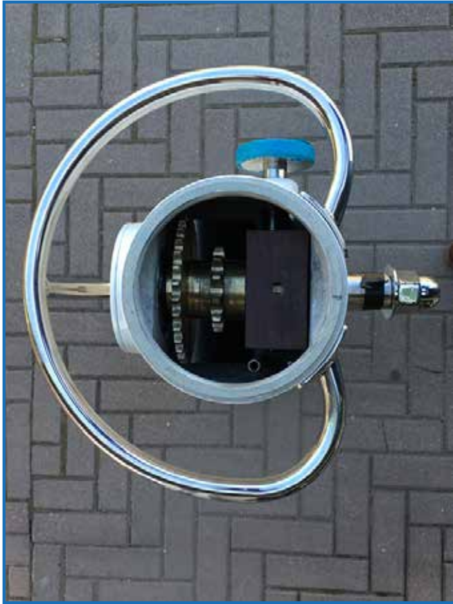
22 - Steering pedestal, aluminum, with originally mounted double crown, for steering chain and Neco autopilot chain
