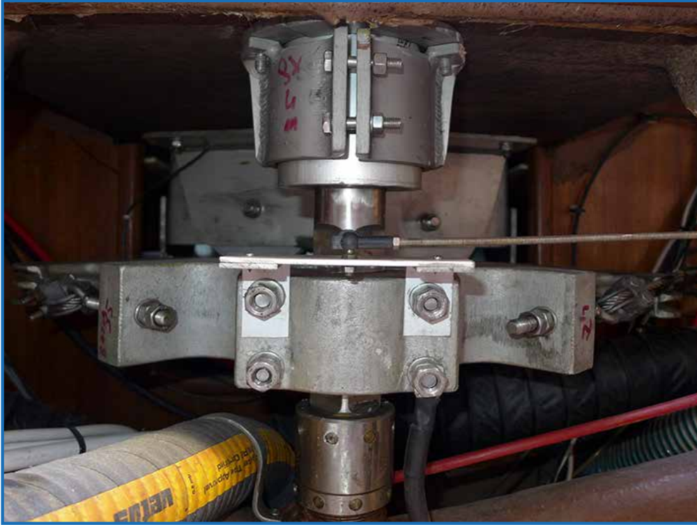
27 - Rudder stock, with quadrant and band packing gland
