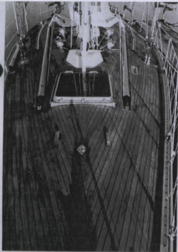
Meticulous teak journey on deck is attention-getting display of Finnish craftsmanship. Two spinnaker poles have slotted storage areas.
