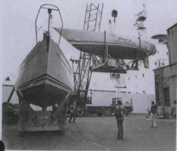
Unloaded in Vancouver harbour, Trumpeter shows hull lines to longshoremen. She has fairly long fin keel, for good lift, a skeg with large rudder.
