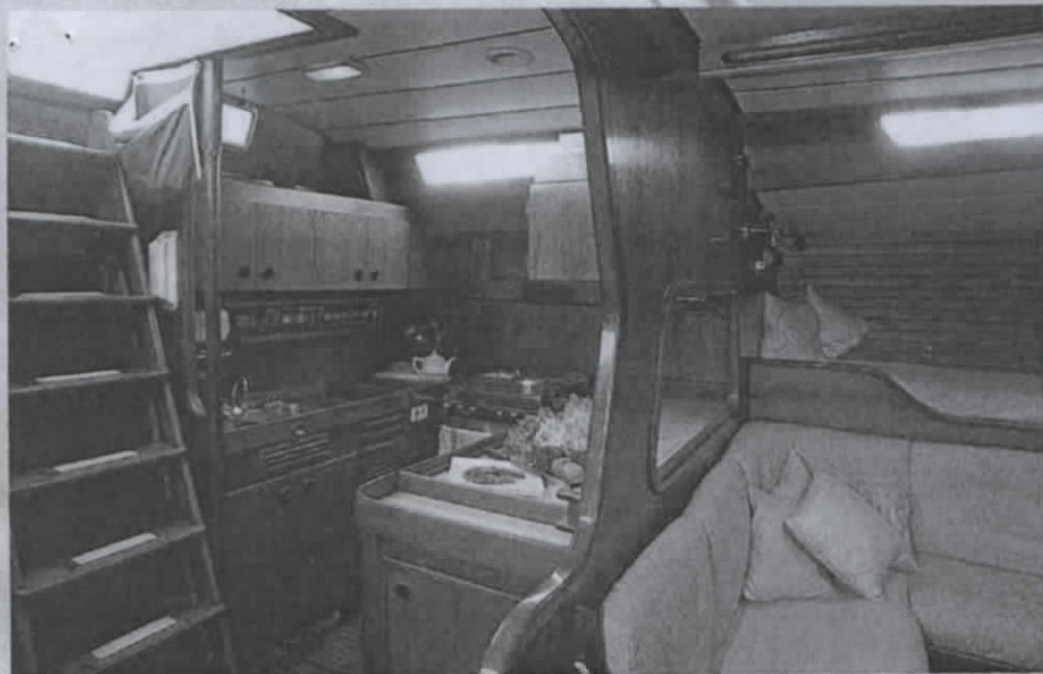
Saloon of Beija Flor showing the impressively roomy galley. A cut out in the bulkhead allows access to the saloon table
