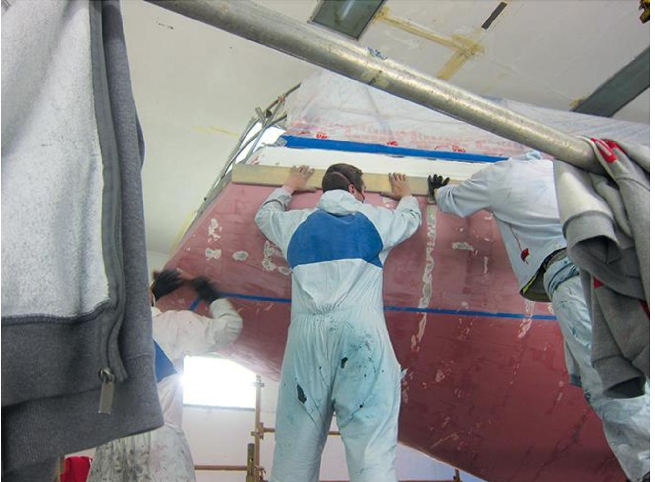
Shipwrights used templates from the line plan to build up and fair the hull
