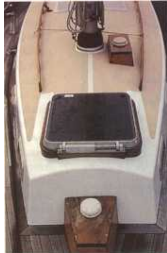
Forehatches and crazed, split coachroof ports are among the first items to replace. A Swan 36 (left) about to undergo a refit and (right) Bramble's reconditioned coachroof with new forehatch ports and varnished brightwork
