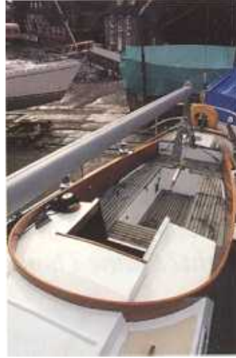
Cockpits before and after. Bramble (left) had her decks laid with teak, all other surfaces painted and brightwork brought up to tip-top condition. Right, a tired Swan 36 cockpit about to be refurbished
