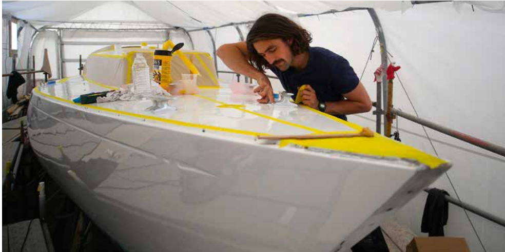
Above: George Maisey fits the new foredeck cleats after the paint job. Left: Harry installs new cabin windows. The old Perspex windows were replaced with polycarbonate
