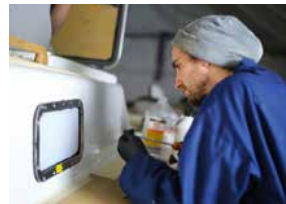
Above: George Maisey fits the new foredeck cleats after the paint job. Left: Harry installs new cabin windows. The old Perspex windows were replaced with polycarbonate
