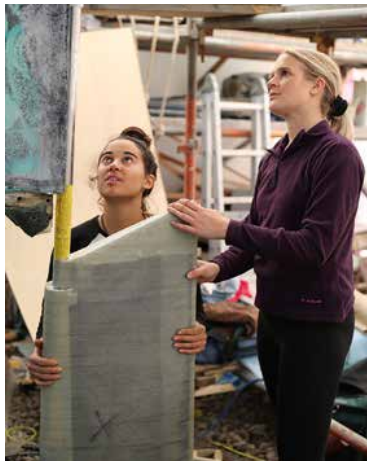
Above: Chloë and Bethany Allen line up the rudder stock
