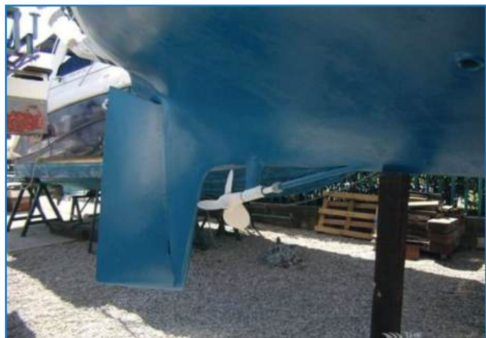
3 - Typical Skeg Hung Rudder Configuration
