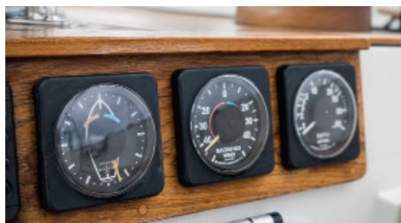
Only simple, non-interfaced wind instruments are allowed in the Ocean Globe Race, with no large on-deck repeater screens
