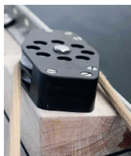
Genoa blocks were refurbished: the refit has focussed on upgrading tracks, blocks and deck hardware to ocean specification
