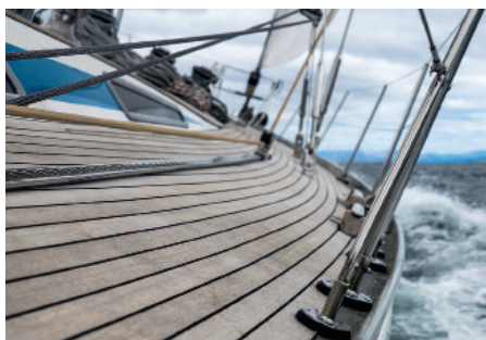
Evrika has classic teak decking – entrants in the Ocean Globe Race must also create room for hi-vis fluorescent areas on deck for safety
