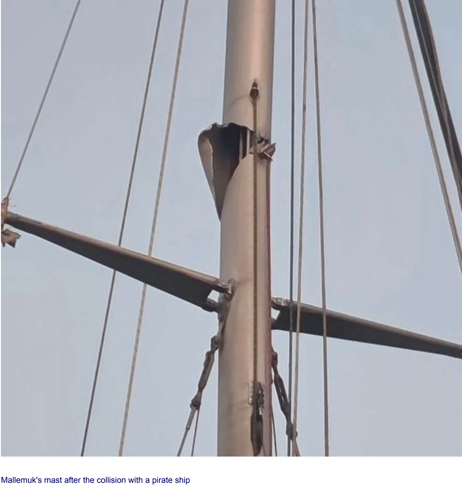
Mallemuk's mast after the collision with a pirate ship
