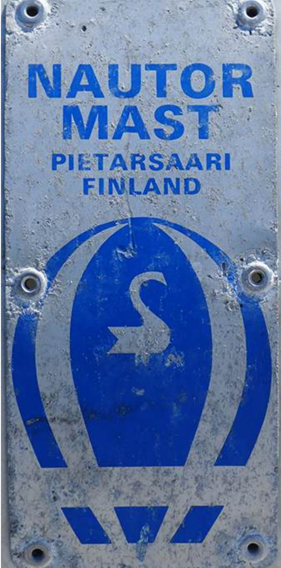
...before installing back in place the boom vang plate after everything was carefully tested the plate was removed once again (as all other mast fittings), the mast sandblasted and finally painted with awlgrip
