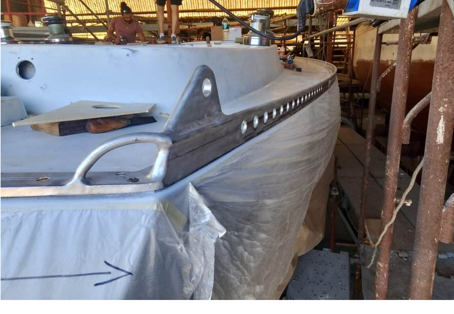
The amazing brand new aluminum toerail, which production was dismissed by the yard, was produced by the owner of S&S Swan 44/016, who has a fundry in Milan (Fondena Battaglia)
