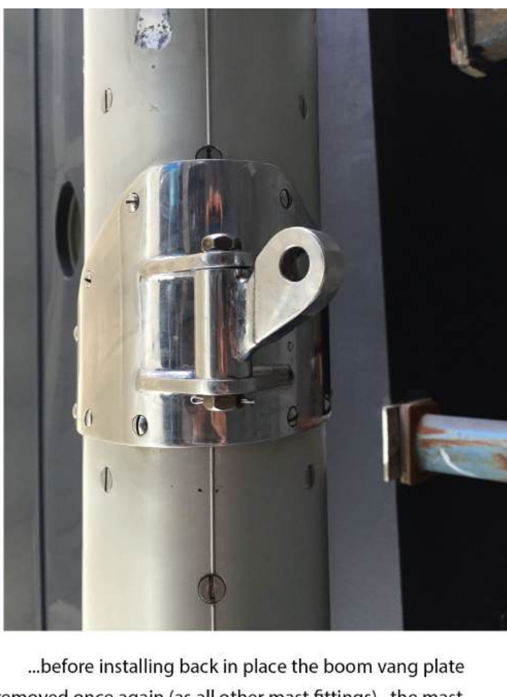
...before installing back in place the boom vang plate after everything was carefully tested the plate was removed once again (as all other mast fittings), the mast sandblasted and finally painted with awlgrip
